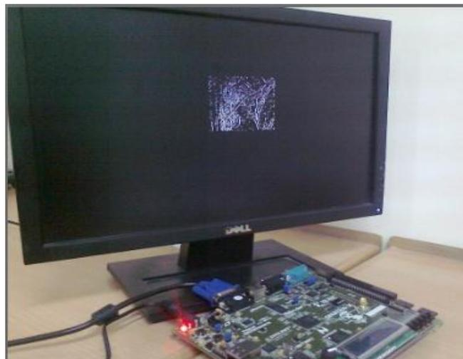
**Figure 4.1 Vga interface of canny edge detection algorithm on FPGA**
